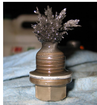
Figure 2: Countershaft Bearing Failure
