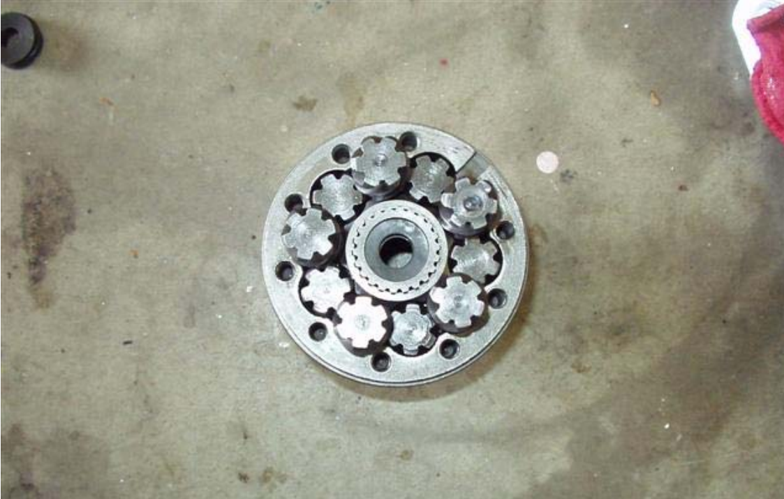
Step 3: Place the thick gear over the washers (it will stick up past the top of the inner retainer if assembled properly to provide preload)
