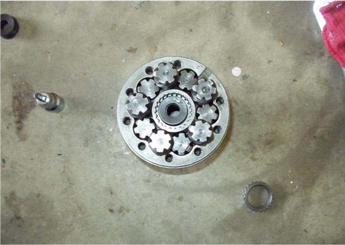
Step 3: Place the thick gear over the washers (it will stick up past the top of the inner retainer if assembled properly to provide preload)
